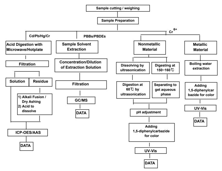
The samples were dissolved totally at the acid digestion step of the above flow chart for Cd,Pb,Hg Section Chief: Timothy Jeon
